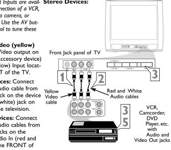
Audio and Video Front Inputs are avail- Stereo Devices: Aable for a quick connection of a VCR, to playback video from a camera, or attach a gaming device. Use the AV button on the remote control to tune these inþuts.
