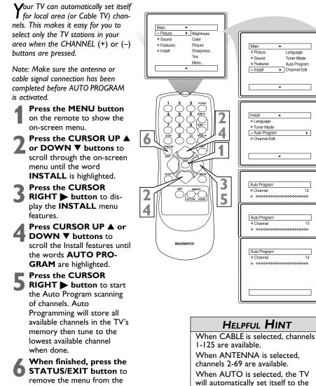
correct mode based on the type of signal it detects when the AUTO PROGRAM feature is activated.
